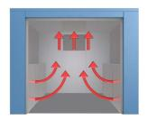
**Dual Airflow:** Hot air is supplied from both side walls and returned through a top plenum. This is the most versatile and common airflow configuration for batch ovens. However, the configuration of the parts being heated must be considered. There must be adequate space around the parts or openings through the parts to permit air to flow to the top return plenum.
